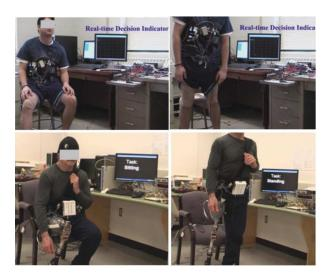
Fig. 6. Real-time testing of the designed NMI prototype on one patient with transfermoral amputation (lower two photos). Upper two photos show our experiments on an able-bodied subject.
